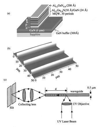
FIG. 1. (a) Schematic diagram showing the waveguide structure fabricated from AlGaN/GaN MQWs. (b) Atomic force microscope (AFM) image of the waveguide sample. Each waveguide has length 500  $\mu$ m and width 0.5  $\mu$ m and the spacing between them is 15  $\mu$ m. (c) The schematic diagram for the time-resolved PL measurement setup. The value d, measured from the edge of the waveguide closest to the slit, defines the position of the focused laser spot on the waveguide.
